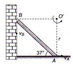
Velocity of end A,  $\vec{v}_A$  is horizontal, while velocity of the end B,  $\vec{v}_B$  is vertical downward. For finding the position of instantaneous centre of rotation. Drop perpendiculars to the directions of  $\vec{v}_A$  and  $\vec{v}_B$  at points A and B respectively. The intersection point I be the instantaneous centre.
