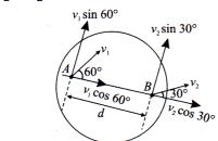
$$\omega_{\text{disc}} = \left| \frac{v_2 \sin 30^\circ - v_1 \sin 60^\circ}{d} \right| = \left| \frac{\frac{v_2}{2} - \frac{\sqrt{3}v_1}{2}}{d} \right|$$
